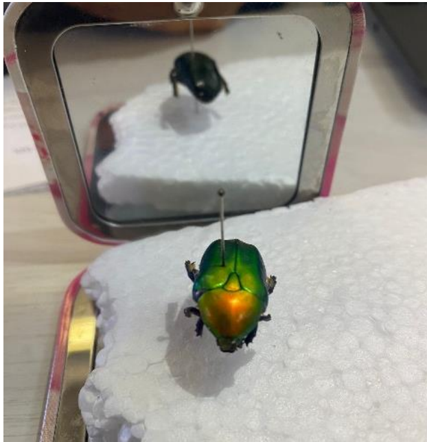
Figure 9: this picture was photographed through left - handed circular polarizer. The color of the Beetle is bright and vivid. Through the mirror it has colorless.
